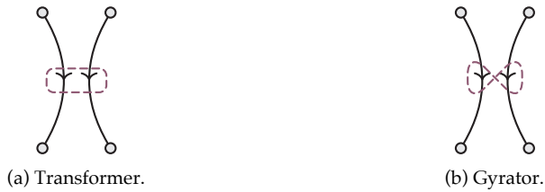
Figure 4.3. Two-port ideal linear graph elements of a transformer (a) and a gyrator (b).
